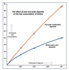
The adhesive properties of unburnt carbon result in a build-up of incombustible solids, ash, and carbon on heat transfer surfaces. The carbon and other deposits act as a thermal barrier, reducing heat transfer and boiler efficiency, and leading to higher stack temperatures in the boiler or air heater. The reduction in heat conductivity relates to a reduction in efficiency, as shown in the graph.
